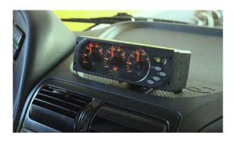
The analog pressure gauges can be embedded in the available space with a DIN format.
