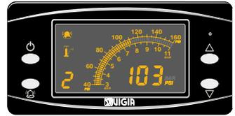
**d) 3 PSI drop takes 2 seconds or less to generate:** Automatic inflation,
