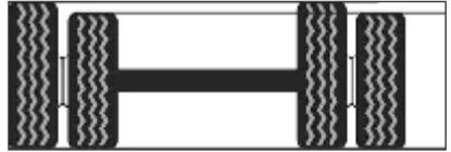
G- Problems in the vehicle suspension, steering or alignment.
