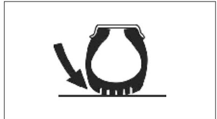
**Important:** According to tire manufacturers' specifications, tire pressure must be calibrated when tires are COLD (allow the tires to cool for 3-4 hours after use). Tire pressure may increase up to 12 % over the "cold" pressure due to rolling resistance when in use. VIGIA will show this pressure increase in the display module. DO NOT BLEED THE TIRES.
