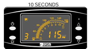
**Manual Mode:** In Manual Mode circuit pressure and air tank pressure (P) can be displayed pressing
