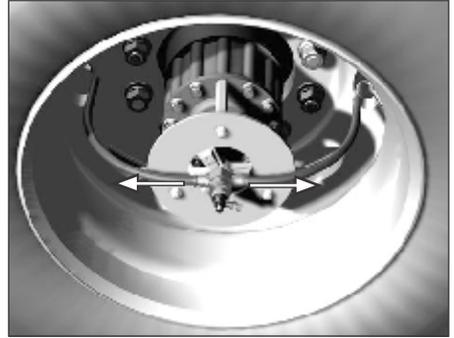
B- Remove the tire taking care of not damaging the rotor.
