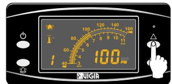
**Important:** The display goes into sequential mode automatically when loss of pressure is detected and it will show the circuit being inflated.
